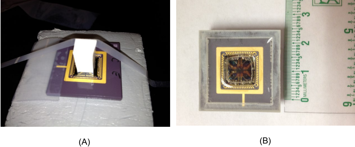
Figure 30: MEA fluid well fabrication using PDMS. (A) a rubber block was used to protect the MEA active area during encapsulation and (B) A finished MEA device with the PDMS containment well and wire-bond encapsulant shown after curing. Ruler shown for scale.
