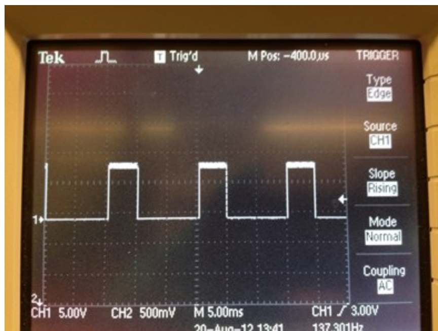
Figure 44: Generated 5 ms optical pulses. Oscilloscope data showing 5 ms optical pulses detected from the 473 nm fiber output of the system. An amplified Si photodiode was used in conjunction with an oscilloscope to display the pulse timing. Each pulse displayed 73.2 \text{ mW} of average power.
